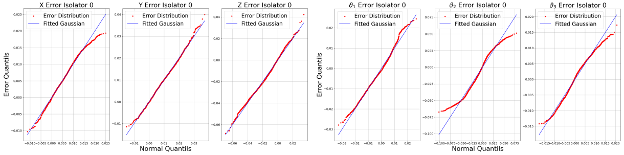
Fig. 5. Componentwise Q-Q plot comparing the error distribution (red) for the translation (left) and the rotation (right) to a fitted Gaussian distribution (blue). The comparison is conducted for insulator 0 and the trajectory depicted in Fig. 4.
