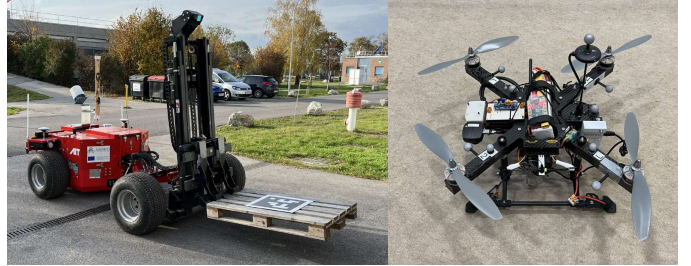
Figure 1. The two different mobile robots used in the real-world demonstration of our anchor initialization method: an automated forklift (left) and a quadcopter (right). The forklift uses two UWB receivers for 3D anchor positioning, as a single tag cannot provide vertical axis information for a ground vehicle. A single UWB receiver is sufficient for the quadcopter, assuming movement along the vertical axis.
