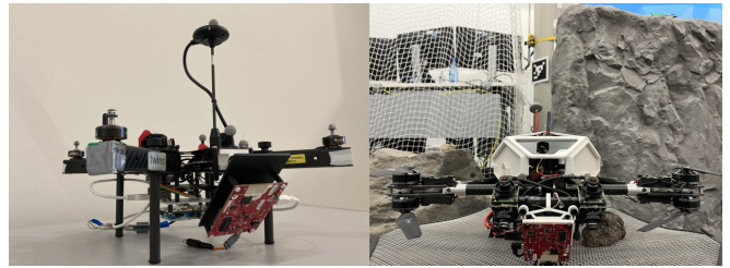
Fig. 1. Experimental platforms used in this work. CNS-UAV on the left and DLR's ARDEA-X on the right. The red chip mounted at 45^\circ inclination on each platform is the TI AWR1843BOOST FMCW radar, which outputs highly noisy and sparse 4D pointclouds (3D points and Doppler velocities).
