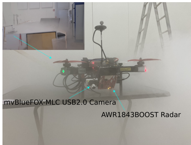
Fig. 1. Experimental platform used in this work with the FMCW radar and camera sensors placed in the take-off position in dense artificial fog used to simulate a disaster site conditions. Note that the camera has been used only for comparison with VIO in the experiments with the artificial fog (see the Subsection V-D).
