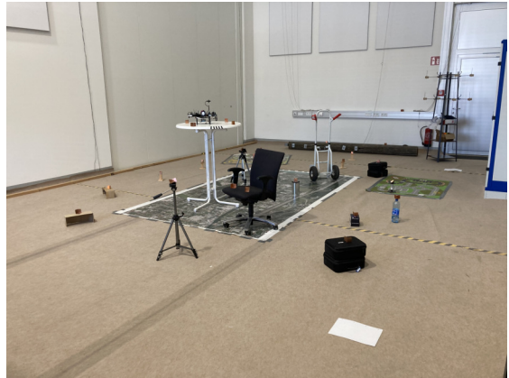
Fig. 4. Indoor space where experiments were performed with reflecting clutter scattered on the scene. The objects were placed randomly and no global position (nor attitude) information of any sort was used in our approach.
