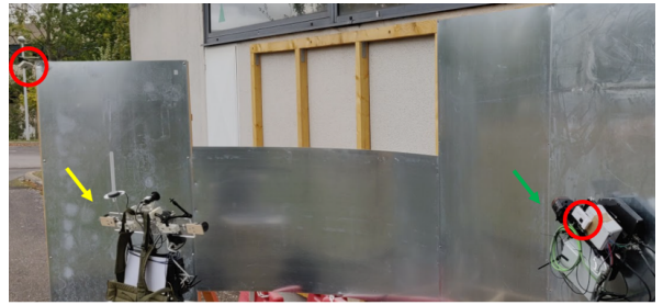
Fig. 2. Magnetic Crawler Robot (green arrow) on a Curved Metal Surface with Ultra-wideband Localization (red circles) and laser (yellow arrow) to track the robot for ground truth.
