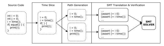
Figure 1: Overview of our approach for detecting time property violations. Time Slice slices the program keeping only the statements that alter and use time variables. Path Generation generates multiple execution paths of the slice based on its control flow. SMT Translation translates each path into SMT constraints. Each model of SMT constraints is fed into an SMT solver to check for violations of time properties in the source code.
