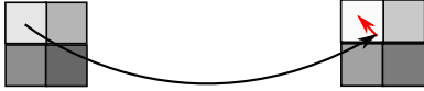
Fig. 3. A pixel intensity value is transferred from the original image position to the predicted image position. As only pixel centers can be destinations, the propagated intensity value is shifted by multiplying the pixel coordinate offset (red arrow) with the gradient.
