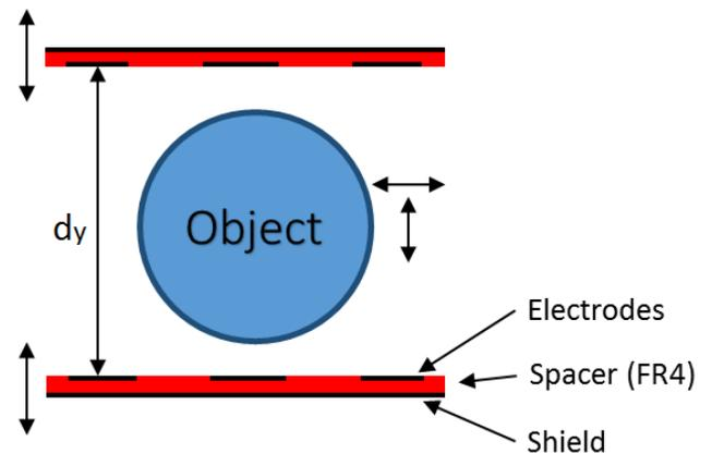
Figure 1. Sketch (2D cross section) of the sensor front end topology comprising two moveable planes with three electrodes on each.
