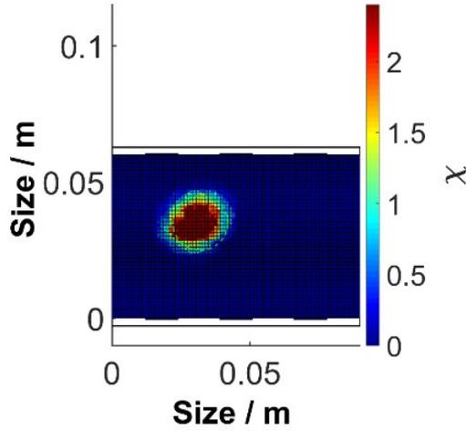
Figure 5. Reconstruction image with a distance of  $d_y = 0.06$  m between the planar sensor front ends. The three electrodes and shield layer are depicted by black lines at the top and bottom of the ROI. The area with the highest susceptibility matches the true position (dashed green line) of the object very well. In addition, no artefacts are visible in the ROI.
