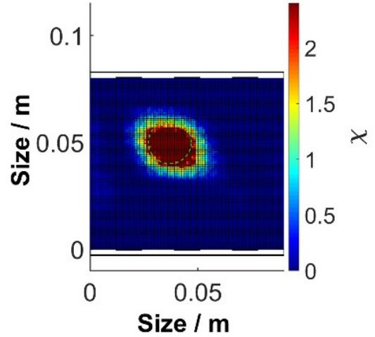
Figure 6. Reconstruction image with a distance of  $d_y = 0.08$  m between the planar sensor front ends. The three electrodes and shield layer are depicted by black lines at the top and bottom of the ROI. The area with the highest susceptibility matches the true position (dashed green line) of the object very well. However, the true susceptibility value does not exactly match the real susceptibility of the object.
