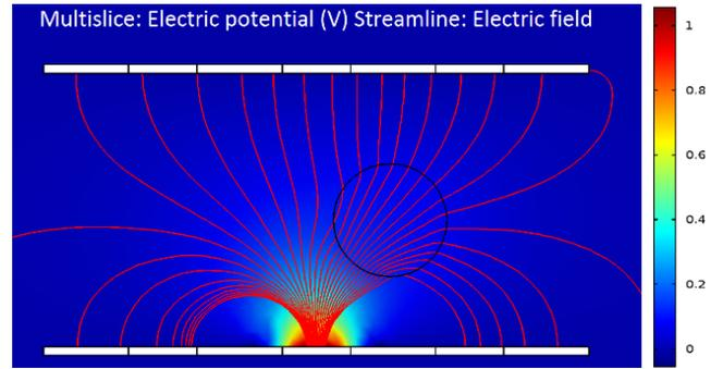
Figure 3. Topview of the 3D finite element simulation of the electric field (red lines) and potential (colorbar) for a sample of the prior distribution. The electric field is distorted by the object depending on its position. The topology is according to the setup given in Figure 1.
