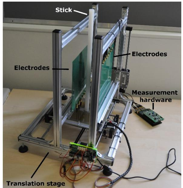
Figure 4. The ECT measurement setup for variable electrode topology comprising the measurement hardware using six input channels, the translation stage to move an object (stick made of erthalon) and the plane sensor front ends consisting of three electrodes and a shield on the back side.
