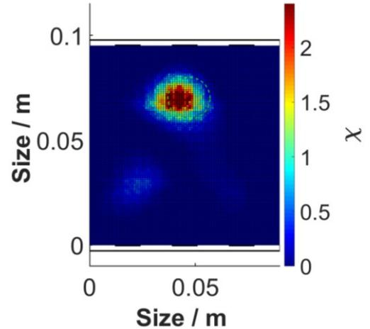
Figure 7. Reconstruction image with a distance of  $d_y = 0.095$  m between the planar sensor front ends. The three electrodes and shield layer are depicted by black lines at the top and bottom of the ROI. The area with the highest susceptibility and the true position (dashed green line) of the object have a close match even if some artefacts occur to the bottom left side of the image.
