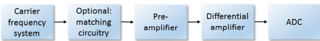
Fig. 7: Block diagram of the analog signal processing chain up to the high-speed ADCs.
