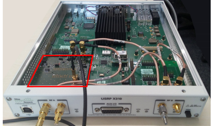
Fig. 4: FPGA platform to be used with specifically designed circuitry as well as developed hardware design and software building blocks. Marked in red is the already attached daughterboard developed for this work.
