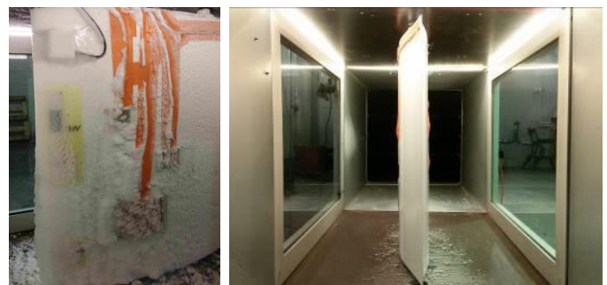
Fig. 3. Icing condition, all three bottom antennas covered with ice (left) Build up of the wing model inside the icing wind tunnel (right)
