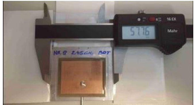
Fig. 2. Dimension of the 2.45 GHz patch antenna with 50 Ohm coplanar semirigid feeding, mounted on a 2mm thick aluminum plate to simulate the influence of the conducting material below the patch
